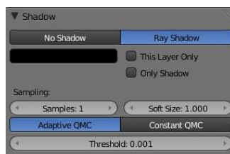
Fig. 2.2095: Point lamp with ray shadows and Adaptive QMC sample generator enabled
